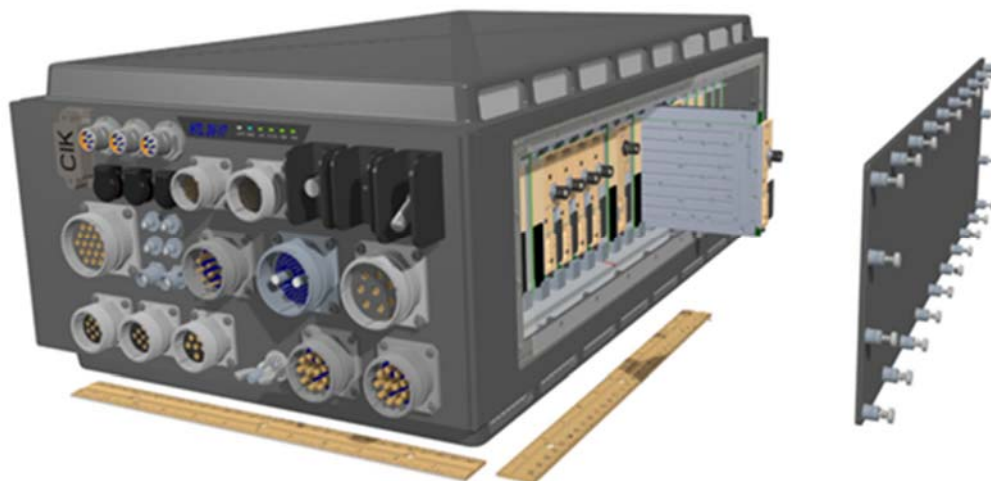
Front panel view of hybrid High Performance Embedded Compute (HPEC) Chassis with 16 channels of Narrow Band Transceivers
