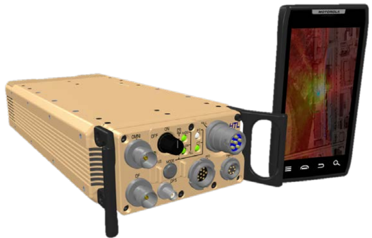
HTLx Core Module in Forced Convection Tactical Housing -Shown with Motorola Razr XT910
